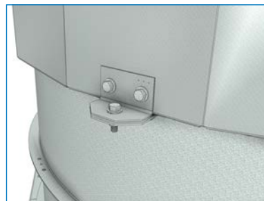
Fasten with M10 hardware.
