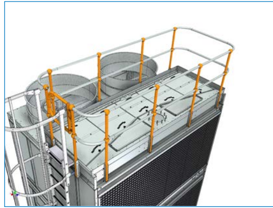
Install all vertical posts.
