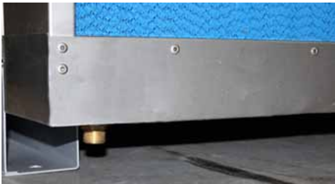
Figure 23: Draining System - outside
