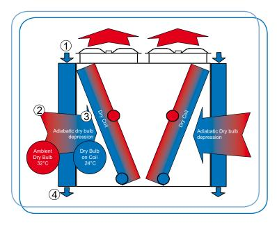
The pre-cooler is constructed in stainless steel, with water distribution piping and a gutter system to drain the water once-through to the sewer ④. Part of the distributed water is evaporated, while the excess water assists in rinsing the pad to keep it free from debris and minerals that would stay behind on the pad after evaporation.
