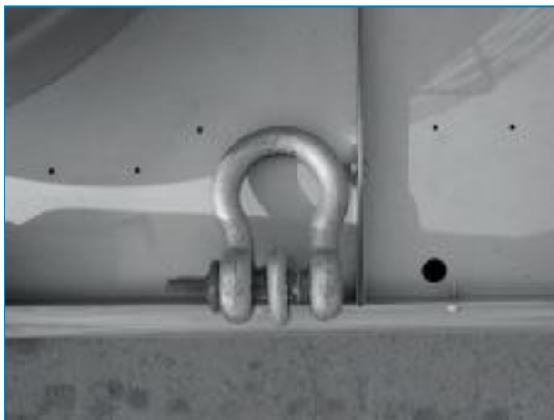
Use shackles (max. Ø 39mm) to lift the unit
