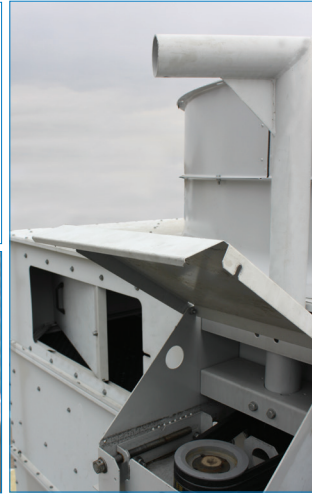
Inward sliding access door. Motor with external adjusters and removal davit*
