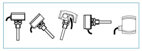
Permitted Positions for mounting VFD sensor
