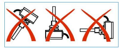
Not Permitted positions for mounting VFD sensor
