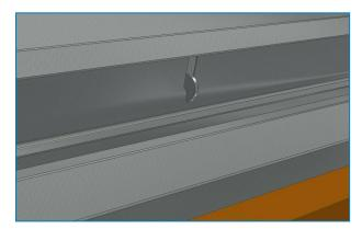
3. Unscrew the flexible sleeve connection by loosening the sleeve clamps. Use a 7 mm spanner or other appropriate tool.
