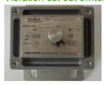
The switch **detects excessive fan drive vibration** caused by or any mechanical fault. Although factory mounted, the switch point is adjusted on-site during installation and start-up.
