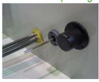
Our factory-installed heaters keep the water temperature at 4°C and act as a simple and economical **anti-freeze measure for the basin water**. The heater package includes the **heaters**, a **thermostat** and a **low level cut out switch** to protect the heaters if the water level declines excessively. Standard electric heaters can handle ambient temperatures down to -18°C.
