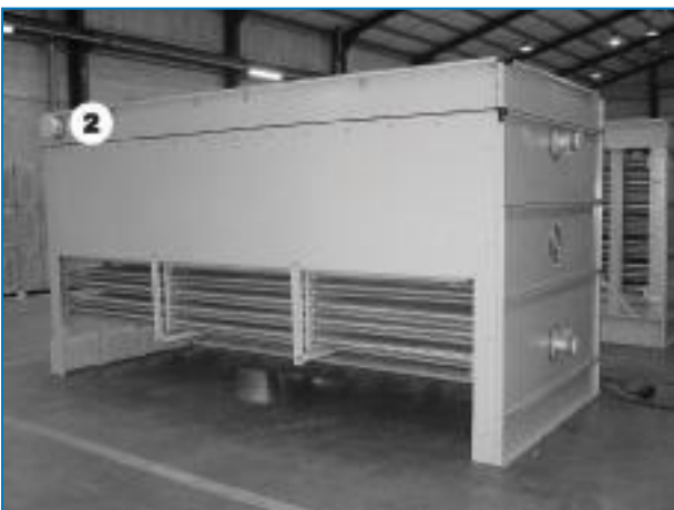
Pump Piping Connection on Coil Section
