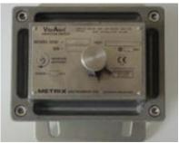
The switch **detects excessive fan drive vibration** caused by fan icing or any mechanical fault. Although factory mounted, the switch point is adjusted on-site during installation and start-up.
