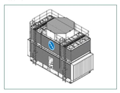
Platforms facilitate **easier** and **safer access** to the **top level** of the unit, making inspection and maintenance easier and conforming to safety standards.
