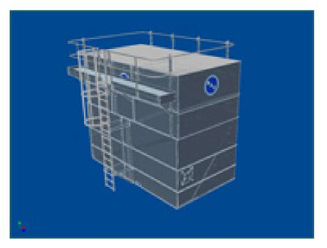
Platforms facilitate **easier** and **safer access** to the **top level** of the unit, making inspection and maintenance easier and are in line with European and South African safety standards.
