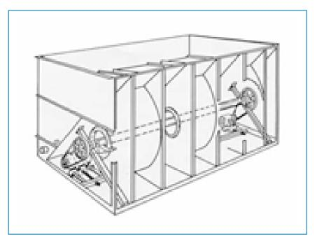
The installation of a Baltiguard® Drive System
